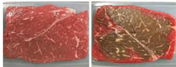
Beef discoloration test - after three days of storage (showing the underside of the meat) (Left) Fresh Master (Right) Unicharm's meat paper product
