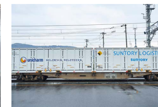
Use of 31 ft large-scale containers also enhances rail transportation [Bringing in 31 ft large-scale rail freight containers]
